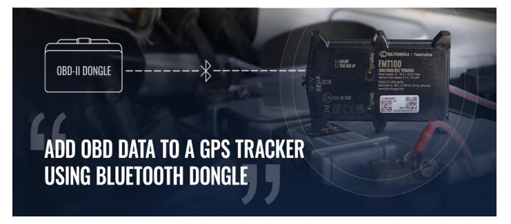
To showcase and explain it, we choose Teltonika SPECIAL category GPS tracker FMT100 model specifically developed for the insurance telematics industry. You can learn more about its use case and benefits here. Additionally, we utilise the onboard diagnostics dongle, the device that plugs directly into the vehicle OBD-II (aka OBD2) port and connects wirelessly to the tracker via Bluetooth connectivity.
